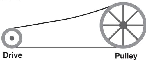
Typically, one rotating shaft serves as the drive and the other rotating shaft serves as the load. An electric motor supplies power to the drive shaft. Pulleys – sometimes referred to as sheaves – can be selected in different diameters. Pulley size differentials can be used to drive the rotating load at a different rpm from the drive shaft. The load can operate at a speed that is the same, or is higher or lower than the drive shaft.
