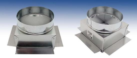
Hercules Industries provides an efficient Square to Round connection piece that is suitable for most HVAC applications. Connects insulated flexible duct or round pipe to a flat surface Can be used to route air from any side of the plenum or a rectangular duct run. Fits most HVAC types for universal application and our manufacturng style with a tacky seal helps create a secure, airtight seal.
