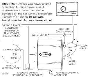
IMPORTANT: When Model 50 current sensing relay is used, wire Model 50 current sensing relay into 24 VAC humidifier control circuit only! Do not install in transformer primary circuit.
