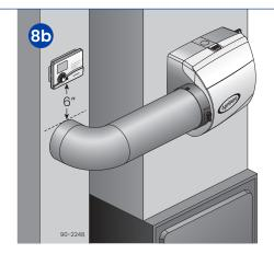
Locate manual or digital humidifier control on the return 6" above the humidifier or bypass duct.
