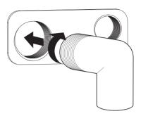
3 Using an approved sealant, insert the PVC pipe into the female end. Condensate drain must be piped to an adequate drain.
