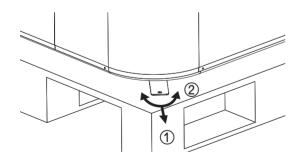
4 Slightly tip the water heater and carefully roll the water heater off the pallet.
