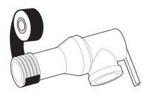
Install the T&P relief valve in the opening marked T&P relief valve.
