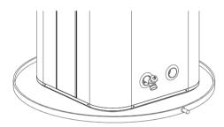
3 Ensure the water heater is horizontal using a spirit level.
