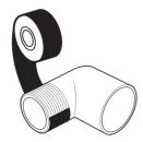
**2** Attach elbow with 3/4" slip &3/4"NPT to the primary drain connection.
