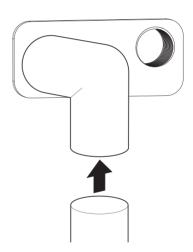
4 Using 1/2" PVC piping, a elbow with 1/2" slip & 1/2" NPT, and an approved sealant, attach the elbow to secondary drain connection and insert the PVC pipe into the female end.
