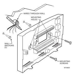
Fig. 6. Mounting the Subbase.
