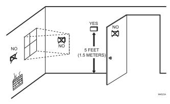
Fig. 2. Typical Location of Thermostat or Remote-Mounted Sensor.
