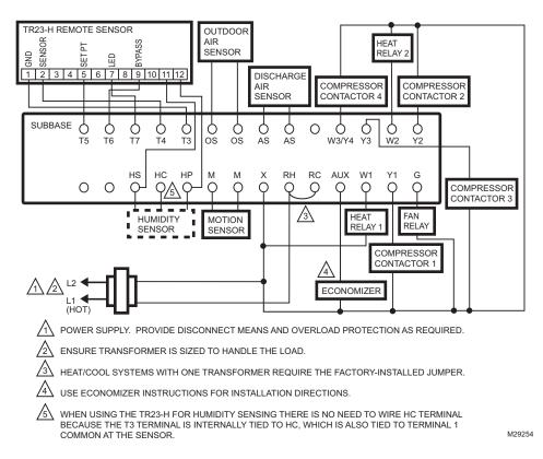
Fig. 15. Typical Hookup of T7351F2010 in Two-Stage Heat and Four-Stage Cool Conventional System.
