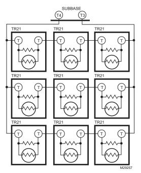
Fig. 5. Nine TR21 Sensors Providing a Temperature Averaging Network for T7351 Thermostat.
