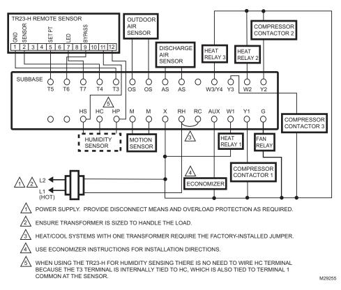
Fig. 14. Typical Hookup of T7351F2010 in Three-Stage Heat and Three-Stage Cool Conventional System with One Transformer.
