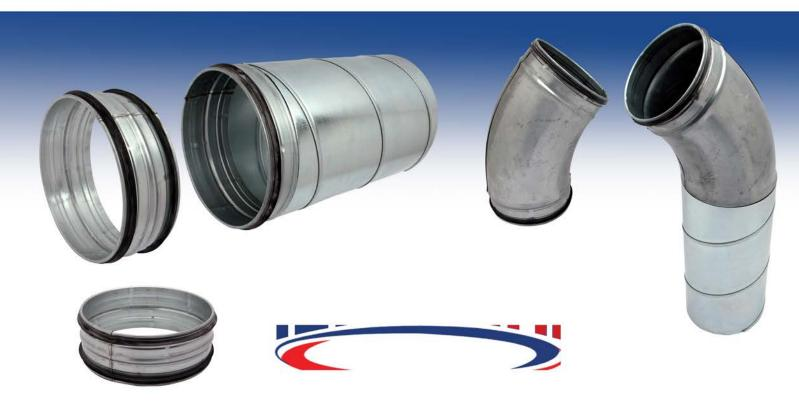
HercSeal gasketed spiral duct fittings are constructed from galavanized steel meeting spec ASTM A-653 (Lockforming quality). They feature a double legged gasket that creates an airtight connection when slipped into the spiral pipe.
